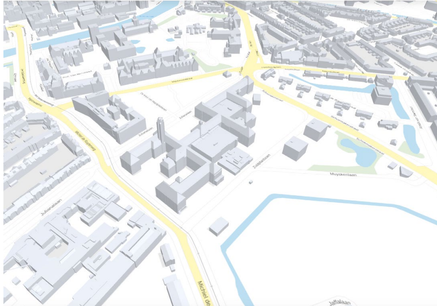
Figure 2 Example of 3D city model utilized a projected CRS (EPSG 7415)
