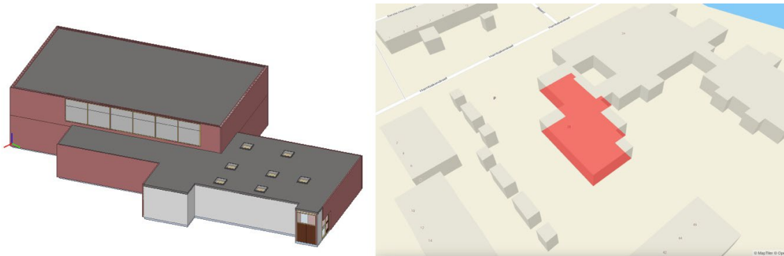
Figure 8 3D view of a georeferenced BIM model (left) and its visualization on the map (right)
